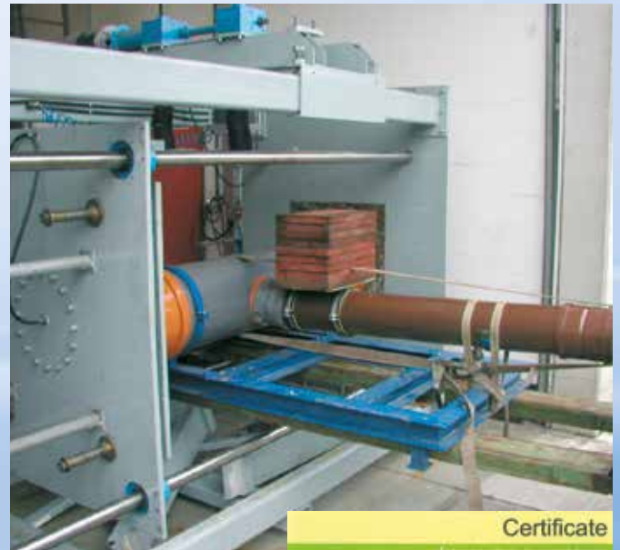
Test set-up for shear loading test
